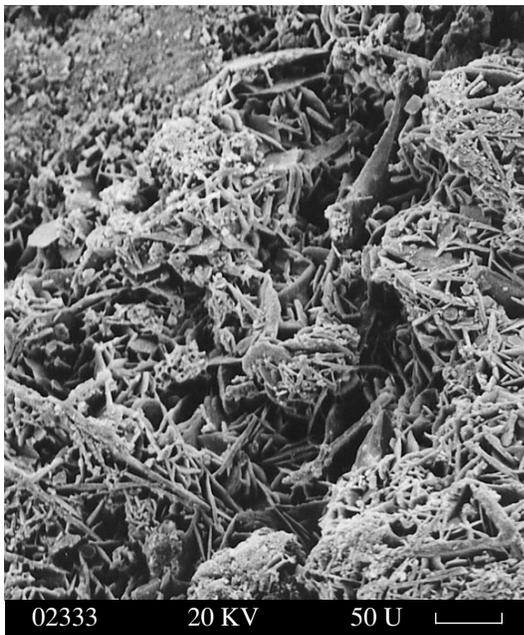
**Fig. 1.** Scanning electron micrograph of a black incrustation with gypsum crystals and dust particles on the marble surface.
